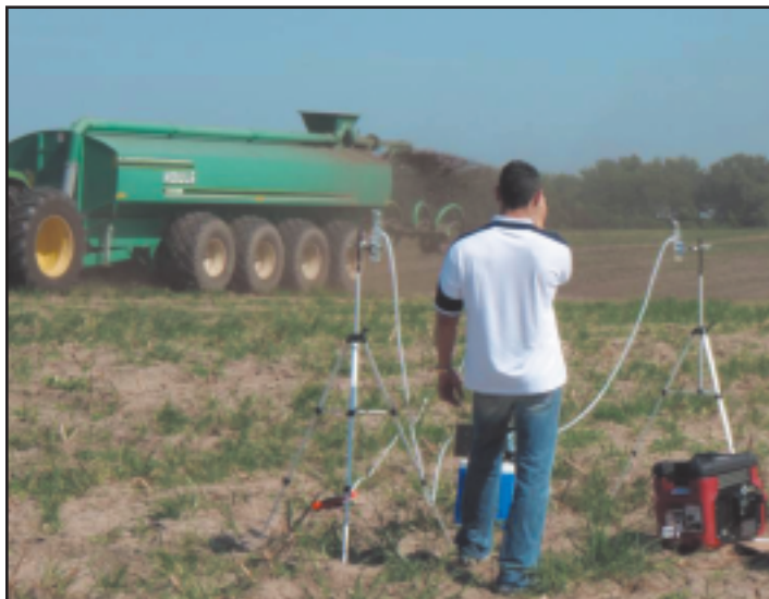
FIGURE 3: Bioaerosol Sampling during Surface Land Application of Biosolids {Field C}
