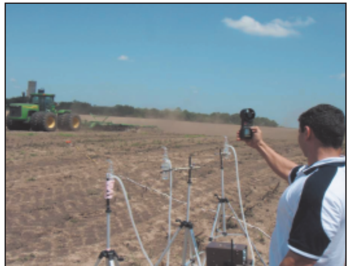
FIGURE 4: Bioaerosol Sampling during Disking Operation (1-Day) [Northwest] {Field C}
